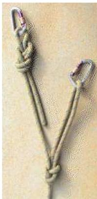
But, as before, if we make the long leg the doubled one, the load is better equalised between the points. In this case, at a 12 kN fall load, the short leg reaches 6.4 kN and the long leg 6.1 kN. This is a 32% decrease maximum force! And this is achieved by simply using the same basic rules, to double the longer leg and a single rope on the shorter leg.
