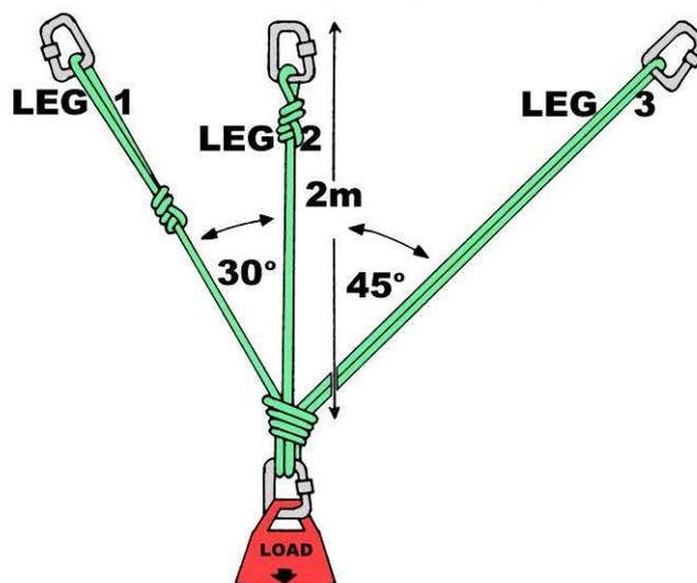
Each placement in the optimised situation carries about 7.8 kN. **This means the system can carry a total load of 70% more** before the force on the centre leg is the same as it was with our original threading sequence! Very little effort gives us all this extra load capacity. A 70% increase in the factor of safety is not to be sniffed at – especially if you happen to be the dope on the end of the rope.
