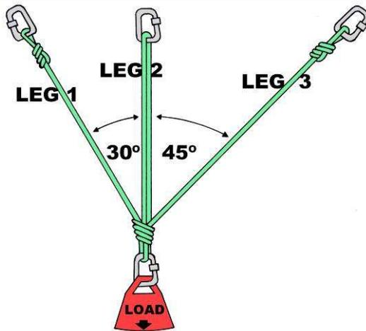
So the strongest system is where ALL points carry equal load to the point of failure. This will have the highest possible factor of safety.
