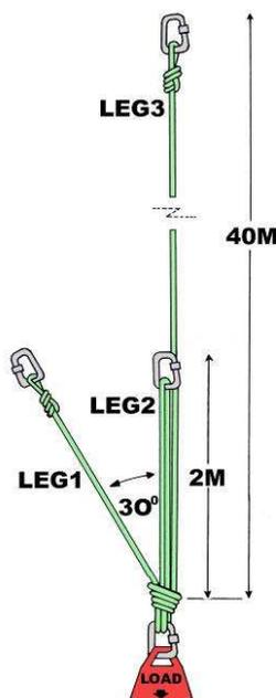
If we let Excel do the calculations again we find the following loads: 5.6 kN, 14.8 kN and 0.4 kN for legs 1, 2 and 3 respectively. In other words leg 3 carries virtually nothing until leg 2 and then leg 1 fails. To carry any load it needs to stretch. Low-stretch rope would need to stretch about 0.7 m to carry its share of the load. Dynamic rope would have to stretch over 4 m. Now it is easy to see why we use low-stretch ropes for rescue!
