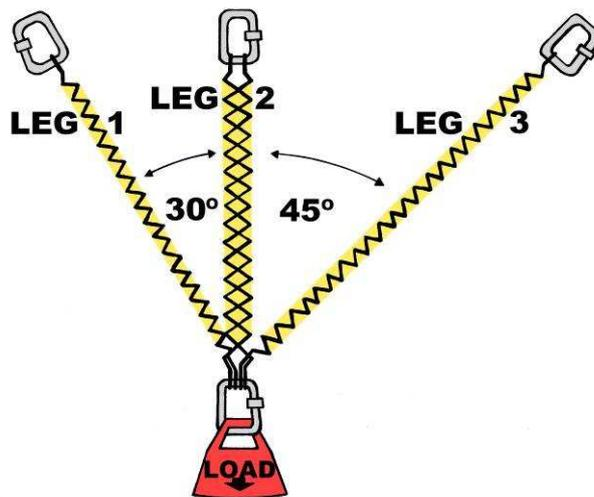
This means that for a typical setup as shown in Figure 2 one gets over three times as much force on the leg 2 placement as for leg 3.
