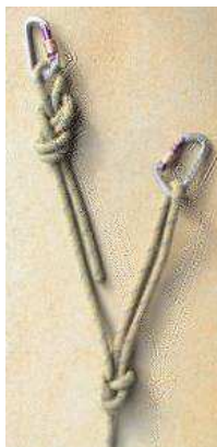
Photo 2 Web Photo to show Equalising Two Anchors
