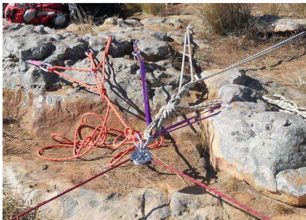
Photo 2 Web Photo to show Equalising Two Anchors
